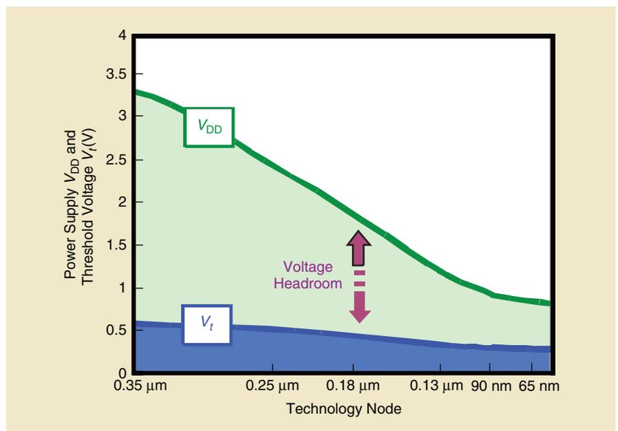
Fig. 1 Downscaling of power supply and transistor threshold voltage in CMOS technologies.
