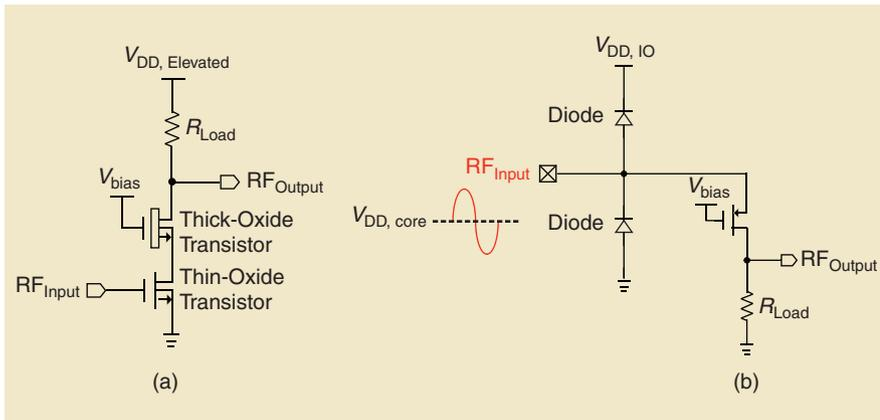
**Fig. 2** RF Amplifier based on (a) a cascode structure with both thick- and thin-oxide transistors, and (b) an open-source-input ESD-protected structure using mixed power supply levels ( $V_{DD, core}$  and  $V_{DD, IO}$ ).
