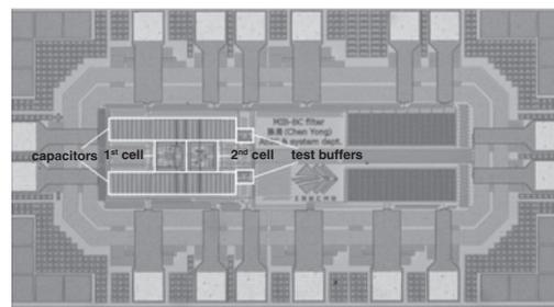
Fig. 2 Chip micrograph of MIB-based filter
