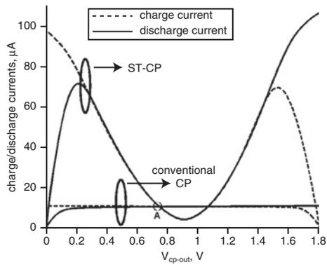
Fig. 3 Charge/discharge currents of conventional CP and proposed ST-CP
