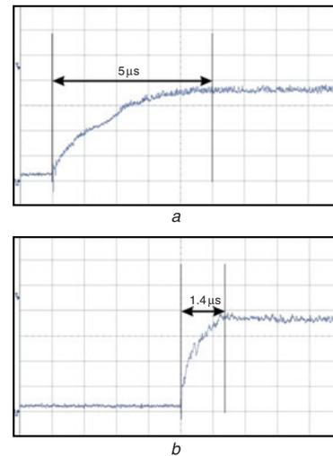
Fig. 5 Measured PLL locking time
