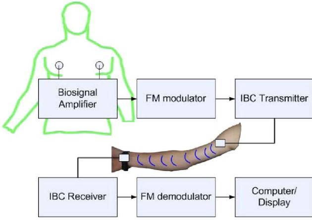
Fig. 2. The block diagram of the system for Electrocardiography signal transmission.
