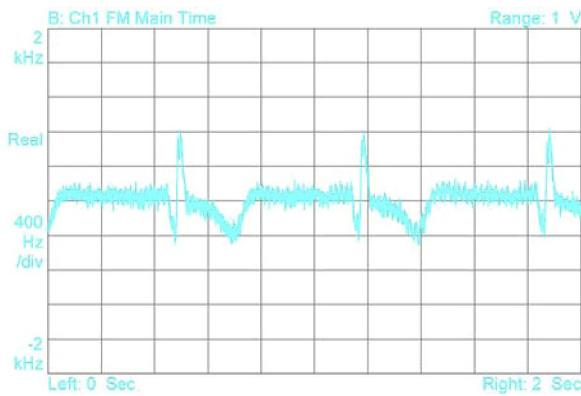
Fig. 4. The ECG signal recovered from the IBC signal received.
