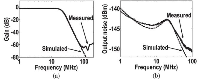
Fig. 9. Measured and simulated (a) frequency response and (b) noise response.
