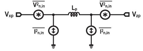
Fig. 3. Noise-equivalent circuit of the FDAI.
