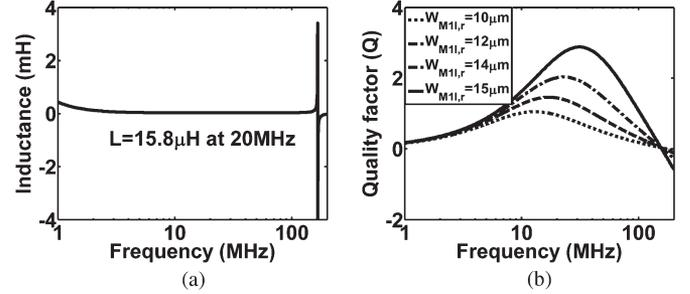
Fig. 4. Simulated frequency-domain behaviors of the FDAI: (a) inductance and (b)  $Q$  factor.
