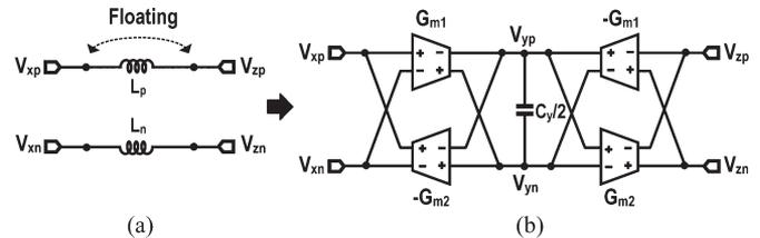
Fig. 1. (a) Floating differential inductor was typically emulated via (b) four  $G_m$  cells and one capacitor configured as a negative-feedback gyrator.
