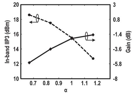
Fig. 7. Tradeoff between gain and in-band IIP3 with respect to  $\alpha$ , which represents the conversion capability from the input signal to the FDAI 1.
