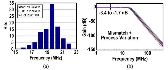
Fig. 6. One-hundred-time Monte Carlo simulation results: (a)  $f_{-3 \text{ dB}}$  variation and (b) the passband gain variation.
