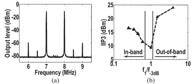
Fig. 10. (a) In-band two-tone test at 7 and 8 MHz (tones at 6.5 and 8.5 MHz are from equipment Agilent E4438C). (b) In-band and out-band IIP3 profile.
