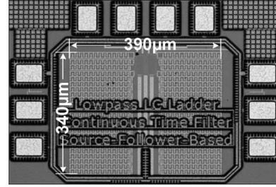
Fig. 8. Chip micrograph.
