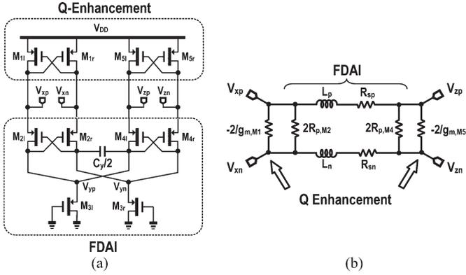
Fig. 2. (a) Proposed transistorized FDAI featuring current-reuse negative  $G_m$  cells for  $Q$  enhancement. (b) Its passive equivalent circuit.
