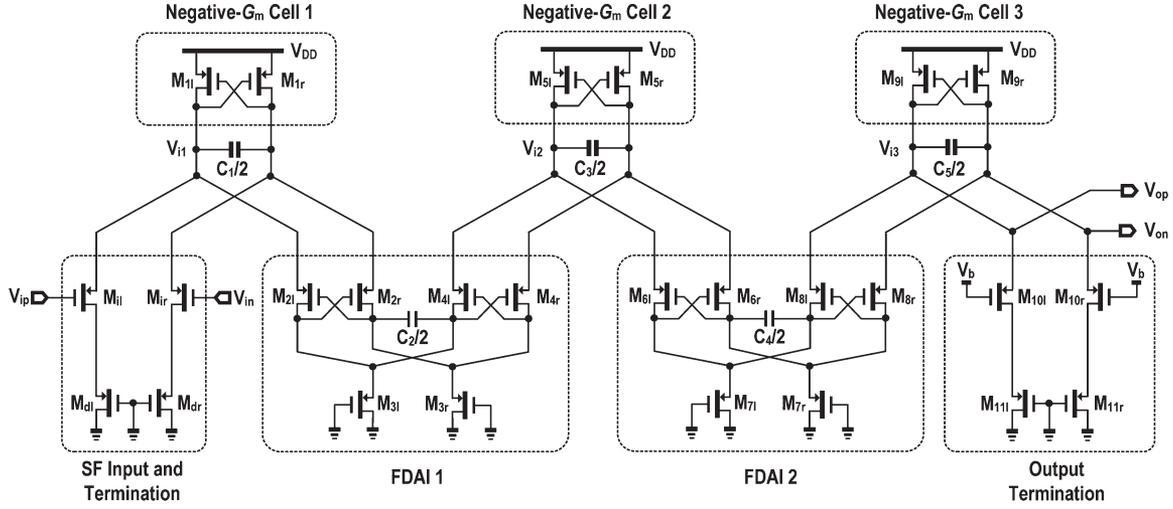
Fig. 5. Realized fifth-order transistorized-*LC*-ladder LPF using SF for double termination and  $Q$ -enhanced FDAs for the floating inductors.
