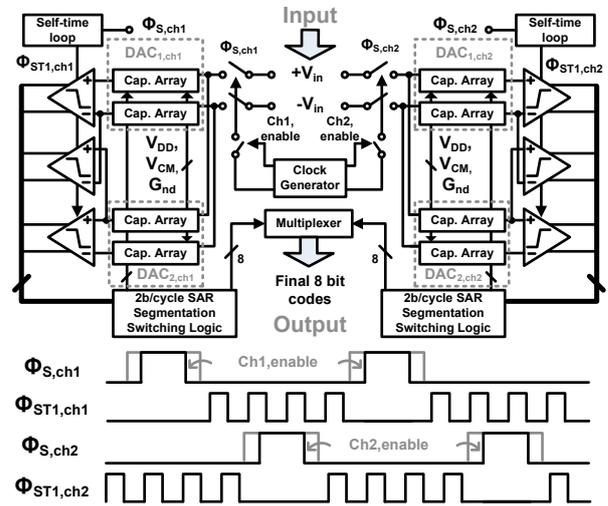
Fig. 1 Overall ADC architecture and its timing diagram.
