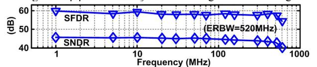
Fig. 6 Measured SNDR and SFDR versus input frequency.
