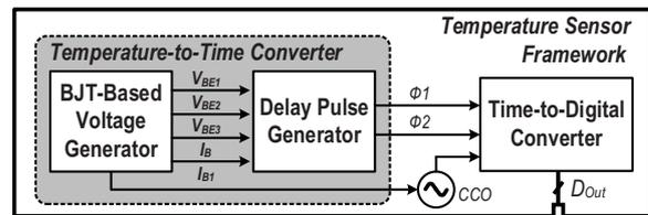
Fig. 1. Block diagram of the proposed temperature sensor.
