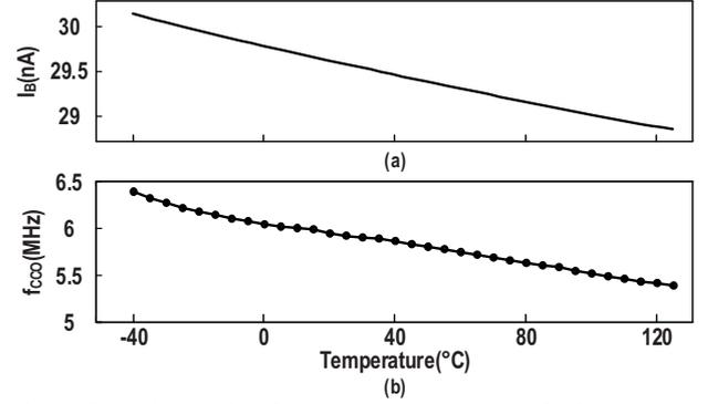
Fig. 5. Simulation results of (a)  $I_B$  vs. temperature; and (b)  $f_{CCO}$  vs. temperature.
