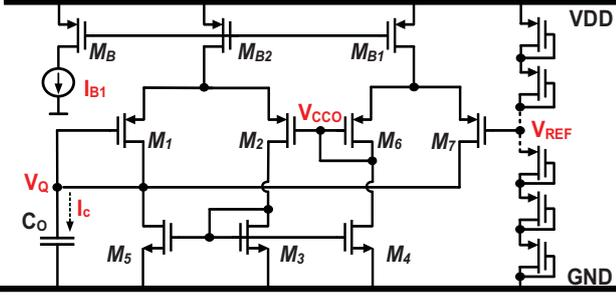
Fig. 4. Schematic of the current-controlled oscillator.
