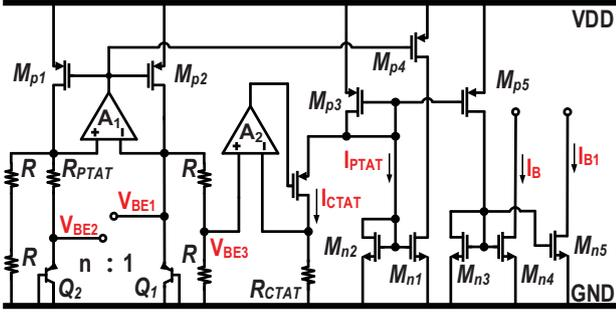
Fig. 3. Schematic of the BJT-based frontend generator.
