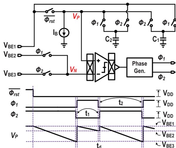
Fig. 2. Architecture of the delay pulse generator.
