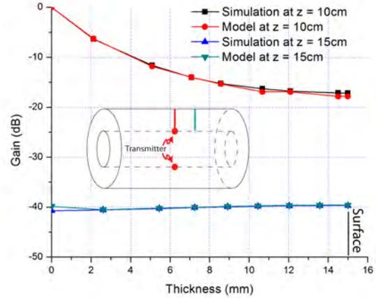
Fig. 3. Signal gain versus outward radial distance
