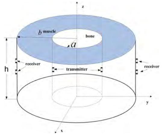
Fig. 2. Cylindrical model for the limb with IMDs
