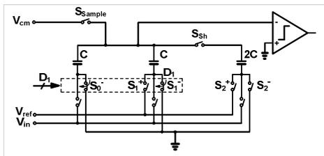
Fig.3. First conversion in the small capacitor (Second step)
