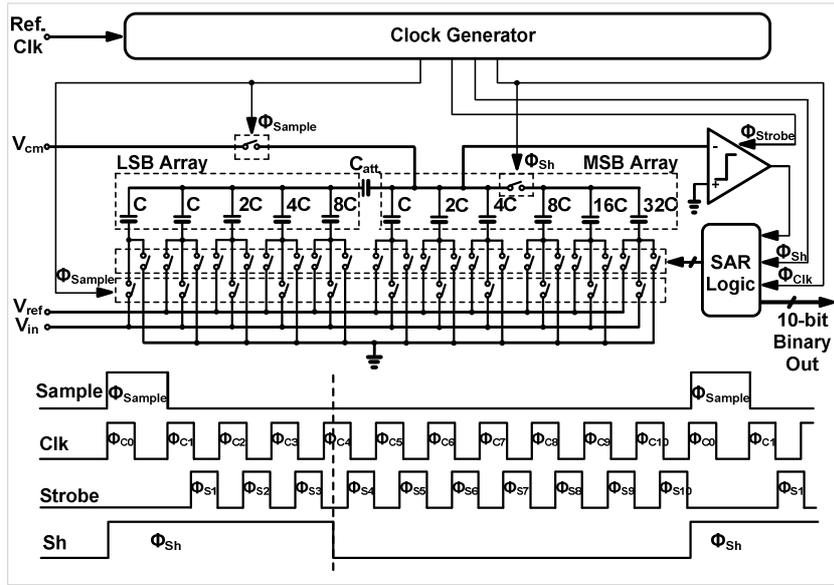
Fig. 2. Proposed ADC circuit and timing diagram
