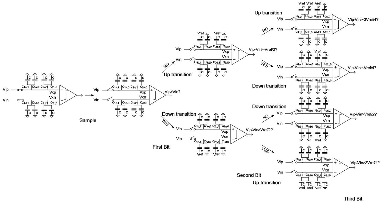
Fig. 2 The single-ended switching procedure of a 3-bit SAR ADC.
