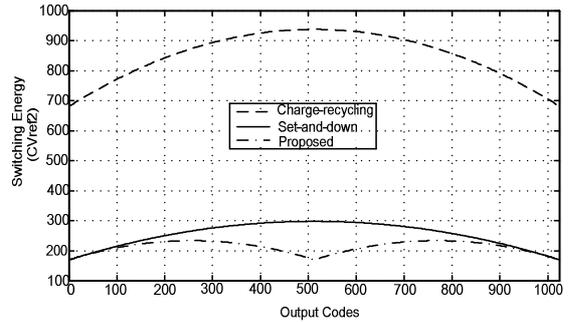
Fig.5 Switching energy versus output code for different switching methods.
