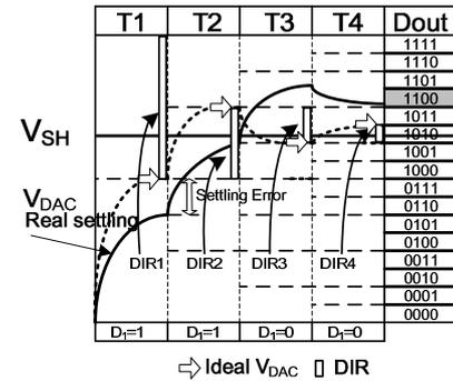
Fig. 1 Example of settling error causing wrong decisions.
