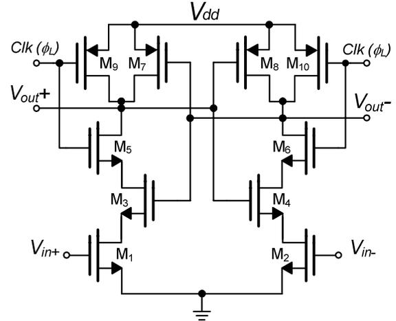
Fig. 6 CMOS implementation of the Latch.
