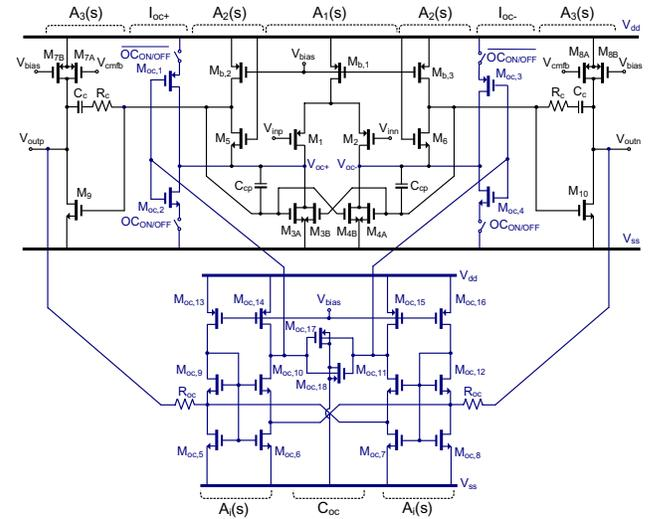
Fig. 5 Full-circuit schematic of the OpAmp and its S-OC.
