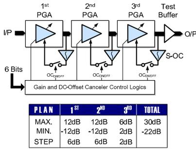
Fig. 6 Implemented PGA and gain plan.
