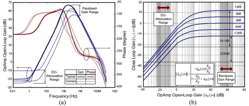
Fig. 7 (a) AC performances of the OpAmp (typical and corners). (b) Closed-loop gains of the PGA versus OpAmp DC and passband gain ranges from Fig. 7(a).
