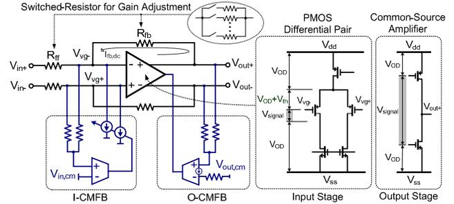
Fig. 1 Low-voltage inverting amplifier with a two-stage OpAmp.
