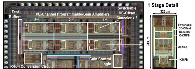
Fig. 8 Chip microphotograph of the PGA (include I and Q channels).
