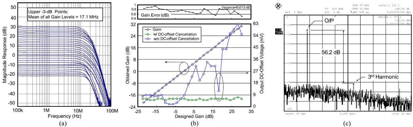
Fig.9 (a) Frequency response at all gains. (b) Designed gain versus output gain, gain error, DC offset with and without DC-offset cancellation. (c) Dynamic-range measurement with 4-MHz single-tone input.
