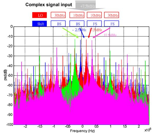
Fig. 8. Post-layout functional simulation in the frequency domain.
