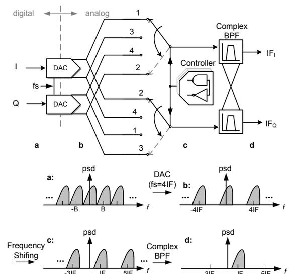
Fig. 2. Detailed D/A interface.
