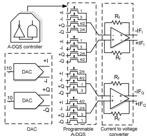
Fig. 4. General circuit architecture of the D/A interface.
