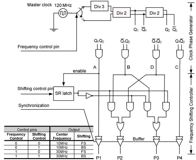
Fig. 6. Circuit diagram of the A-DQS controller.
