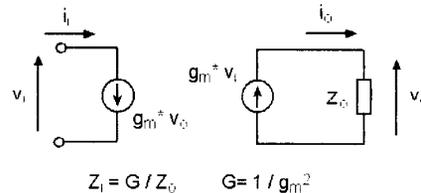
Figure 1. Gyrator working principle.
