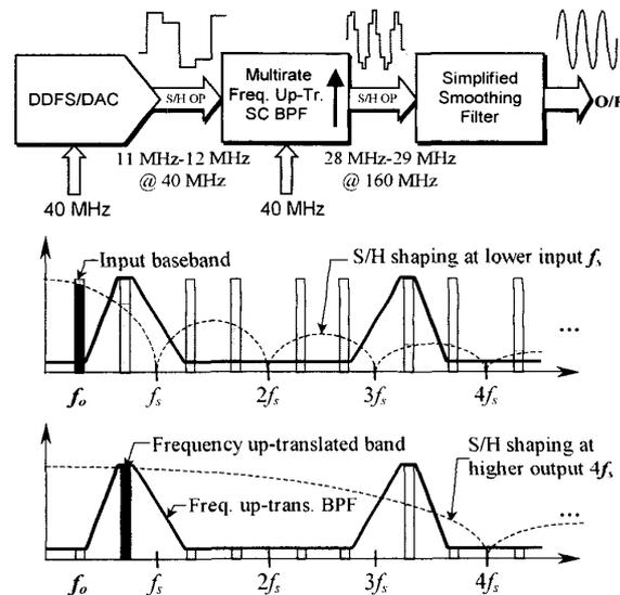
Fig.1 Frequency up-translated bandpass filtering for DDFS systems
