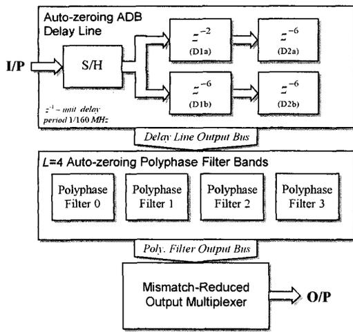
Fig.2 System architecture of the frequency up-translated SC BPF
