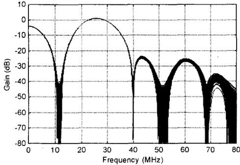
Fig.5 Monte-Carlo amplitude response simulations ( $\sigma_c = 0.7\%$ )
