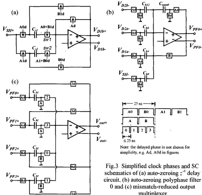
Fig.3 Simplified clock phases and SC schematics of (a) auto-zeroing  $z^{-6}$  delay circuit, (b) auto-zeroing polyphase filter 0 and (c) mismatch-reduced output multiplexer
