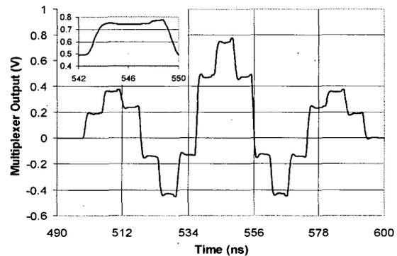
Fig.7 Impulse transient response from layout-extracted worst-case simulation
