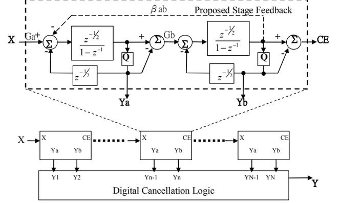
Figure 2. Block Diagram of a Semi-MASH sub-stage.
