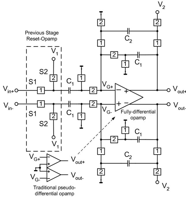
Fig. 2: Low-Voltage SC S/H circuit using fully-differential reset-opamp.
