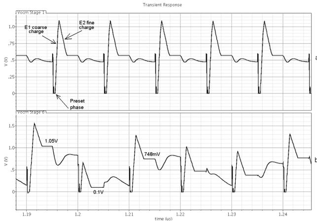
Fig.5 (a) Common mode signals in first stage using CMFB in Fig.2; (b) Common mode signal in 6<sup>th</sup> stage using CMFB in Fig.2
