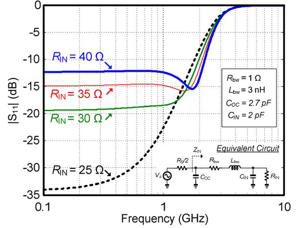
Fig. 3 Input matching design including package effects.
