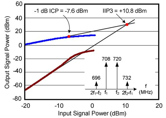
Fig. 6. Two-tone test at 708 and 720 MHz.
