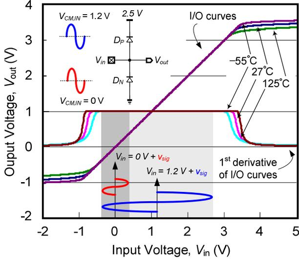
Fig. 2. Diode-clamp I/O transfer curves and their 1<sup>st</sup> derivatives at different temperatures.
