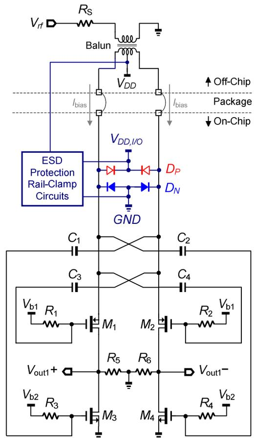
Fig. 1. Proposed PMOS-based open-source-input ultra-wideband LNA with ESD protection.
