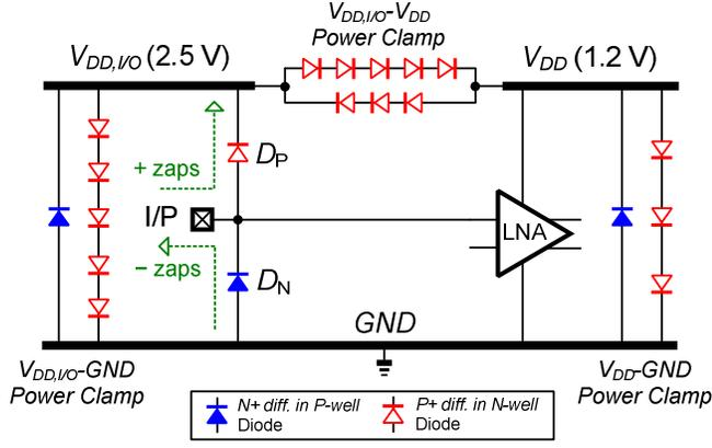
Fig. 4. Mixed-voltage ESD-protection clamps.
