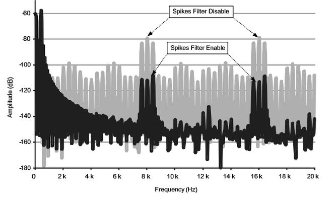
Fig. 5. Chopping spikes filtered by Spike filter
