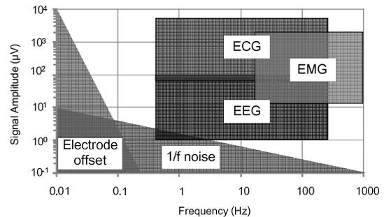
Fig. 1. Bio-potential signals and the nearby contaminating signals
