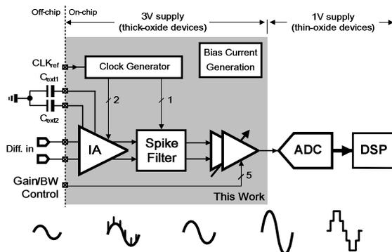
Fig. 2. Proposed bio-potential signals acquisition system.
