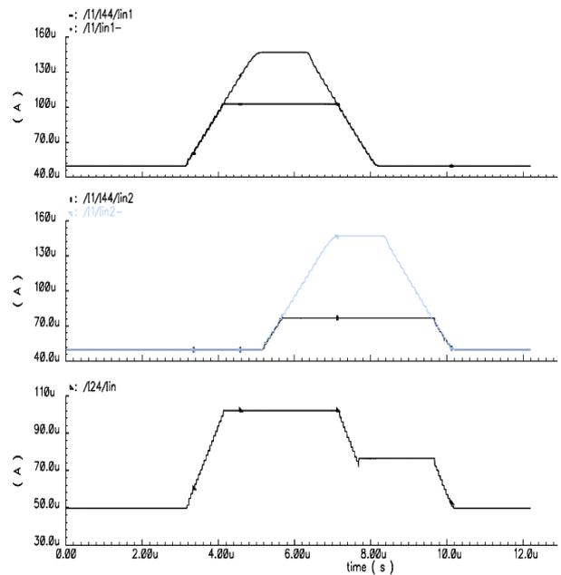
Fig.9 Transient response of truncation process of (a)the first rule, (b)the second rule and (c)the aggregation process of these rules
