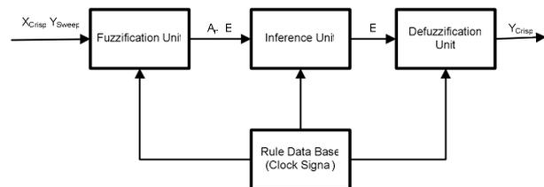
Fig. 1 FLC architecture block diagram.
