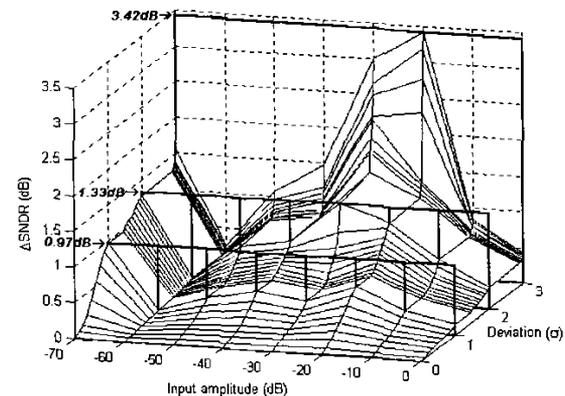
Fig.7 Monte Carlo simulation shows  $\Delta SNDR$  within different deviation  $\sigma$ ,  $2\sigma$  and  $3\sigma$ , where  $\sigma=0.2\%$
