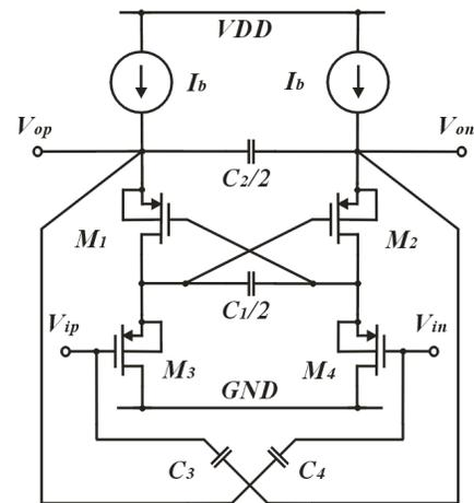
Fig. 1. Proposed SFB low-pass bi-quad cell with poles and zeros.
