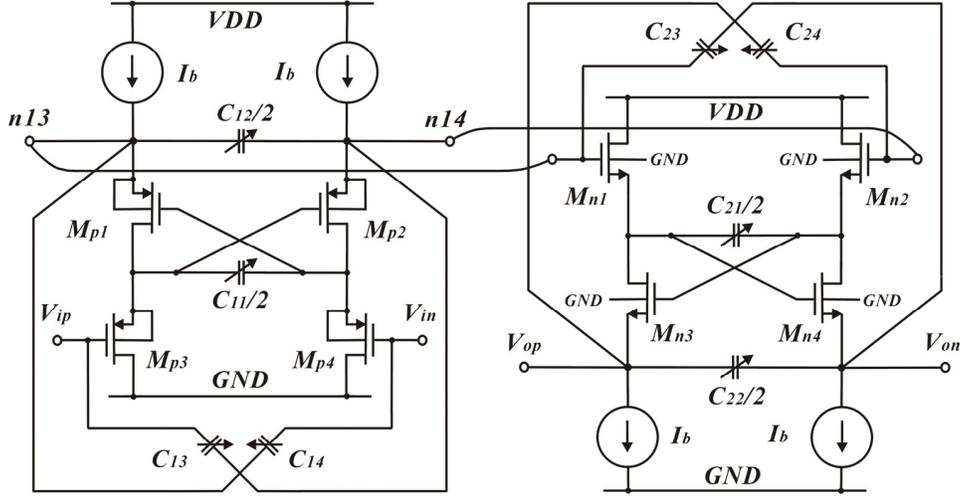
Fig. 2 Proposed and implemented 4<sup>th</sup>-order fully differential SFB active filter
