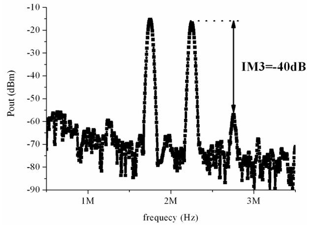
Fig. 5. 2-tone test for In-band IM3 measurement
