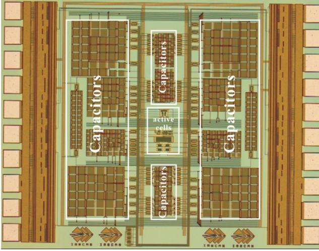
Fig. 3 Die photograph of proposed low-pass filter
