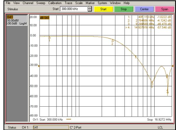
Fig. 4. Measured filter frequency response
