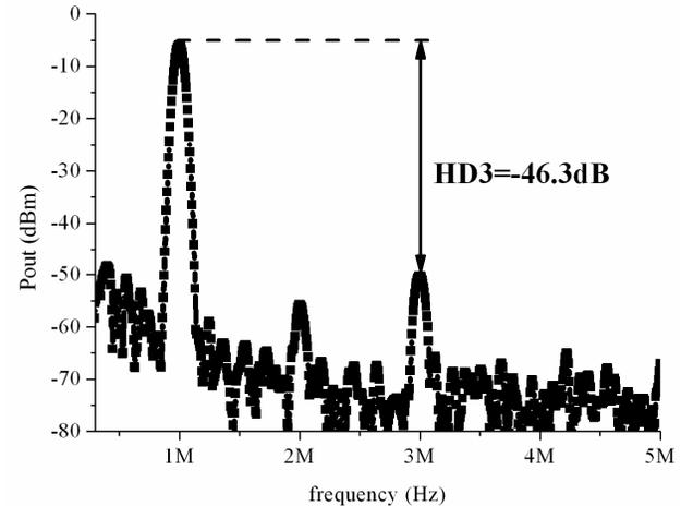
Fig. 6. Single-tone test for In-band HD3 measurement
