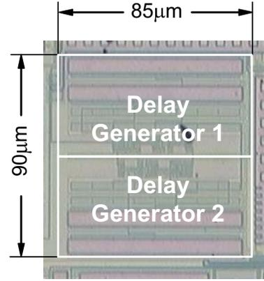
Figure 5: Micrograph of proposed current-controlled delay generator.
