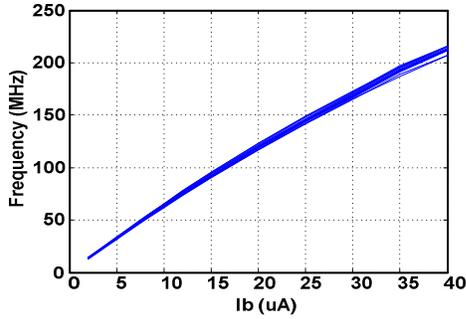
Figure 6: Measured characteristic curves of 14 fabricated samples.
