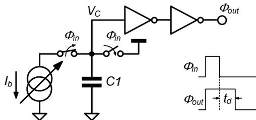
Figure 1: Traditional current-controlled delay generator.
