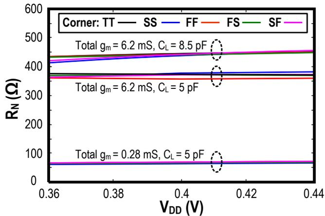
Fig. 5 Simulated  $R_N$  of the XO at 16MHz with different set of  $g_m$  and  $C_L$  versus process variation (5 process corners) and supply voltage ( $\pm 10\%$ ) at 27°C.
