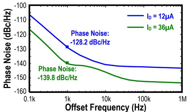
Fig. 7 Simulated PN of the XO versus offset frequency with varying bias condition.
