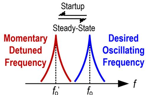
Fig. 1 Illustration of the crystal detuning scheme in the frequency domain.
