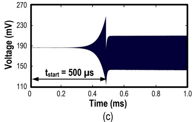
Fig. 6 Startup time of the XO. (a) Without boosting  $g_m$  and  $C_L$ ; (b)  $g_m = 6.2$  mS and  $C_L = 5$  pF in the startup phase; (c)  $g_m = 6.2$  mS and  $C_L = 8.5$  pF in the startup phase.
