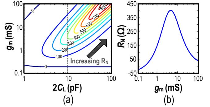
Fig. 3 (a) The contour plot of  $R_N$  against  $C_L$  and  $g_m$ ; (b) The  $R_N$  versus  $g_m$  at  $C_L = 5\text{pF}$ . For both figures,  $f_o = 16\text{MHz}$ ,  $R_f = 2\text{M}\Omega$ ,  $r_o = 5\text{k}\Omega$ ,  $C_s' = 5\text{pF}$ .
