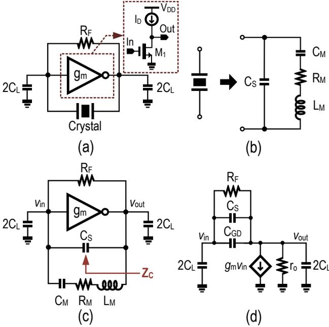
Fig. 2 (a) Schematic of the basic Pierce oscillator; (b) Electrical model of the quartz crystal; (c) Schematic of the Pierce oscillator for deriving  $Z_c$ ; (d) The equivalent circuit for deriving  $Z_c$ .
