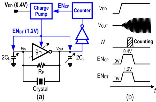
Fig. 4 (a) Schematic of the proposed XO with the control electronics for detuning (highlighted in blue); (b) Timing diagram of the operation of the proposed XO.
