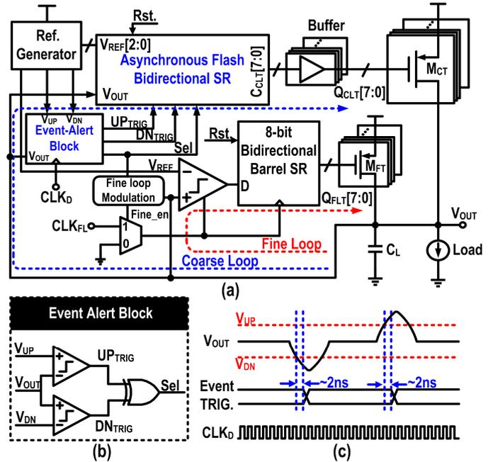
Fig. 1. (a) Overall architecture of the proposed AF-DLDO; (b) the event alert block implementation; and (c) the event trigger timing diagram.
