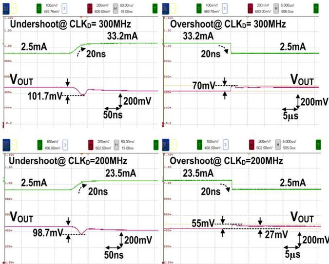
Fig. 5. Measured load transient response with V<sub>IN</sub>=0.5V, V<sub>OUT</sub>=0.45V, C<sub>L</sub>=100pF, and load changes (a) from 2.5mA to 33.2mA within 20ns at CLK<sub>D</sub>=300MHz and (b) from 2.5mA to 23.5mA at CLK<sub>D</sub>=200MHz.
