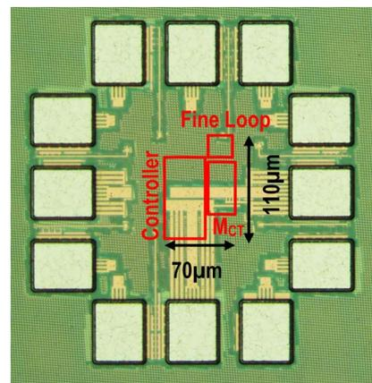
Fig.4. Chip micrograph of the proposed AF-DLDO.
