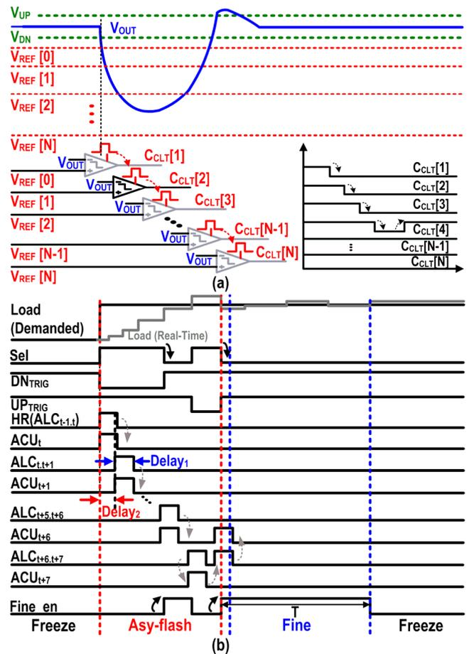
Fig.3. (a) Asynchronous-flash control law (b) Timing diagram under a raising loading step.
