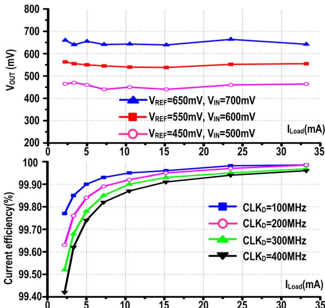
Fig. 6. Measured load regulation with 50mV drop-out voltage (top) and current efficiency (bottom).
