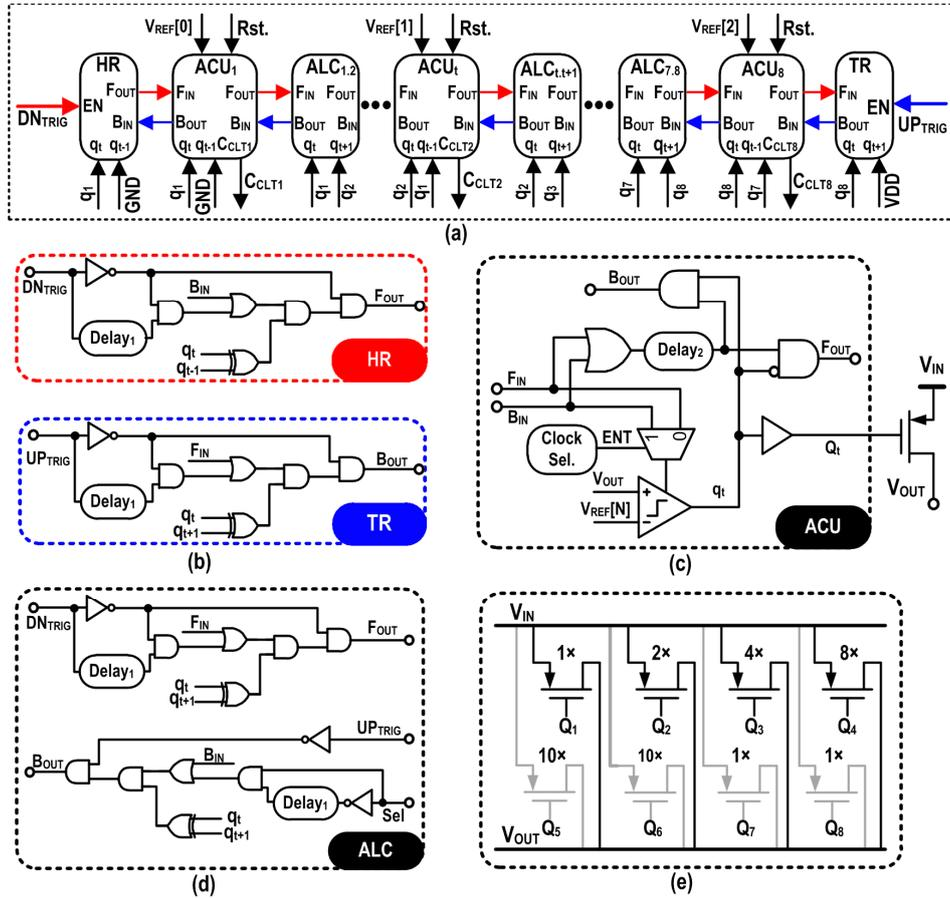
Fig.2. Implementation of the (a) asynchronous flash bidirectional SR; (b) heading reflector (HR); tail reflector (TR); (c) asynchronous control unit (ACU); (d) architectural logic connector (ALC); and (e) power transistor in the AF directed coarse tuning loop.
