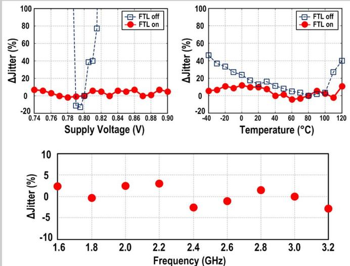
Figure 7.1.5: Measured RMS-jitter variation: <9% against supply voltage and temperature, and <5% versus frequency. REF=200MHz and output at 3.0GHz.
