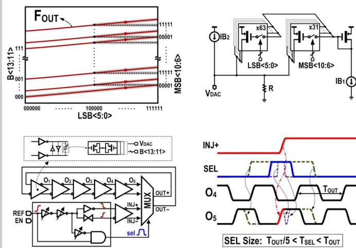
Figure 7.1.3: Upper:  $F_{OUT}$  tuning for seamless decoding and coarse-fine DAC block to optimize area and linearity; Lower: ring-VCO with direct REF-INJ to avoid the divider time constraint and SEL size effect to OUT.
