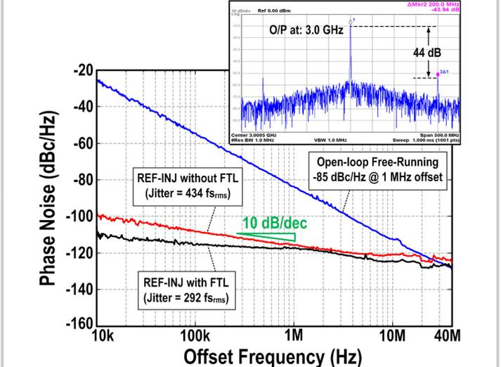
Figure 7.1.4: Measured phase noise: free-running ring-VCO, MDLL with and without the FTL. REF=200MHz and output at 3.0GHz.
