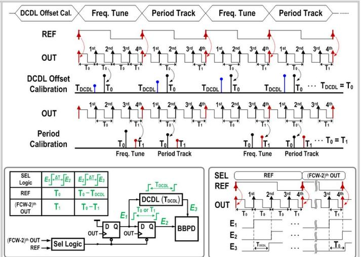
Figure 7.1.2: Timing diagram of the FTL with block sharing in each calibration step. Reusing the same DFF and BBPD logic not only cancels the timing offset and path mismatch, but also saves area and power. FCW=4.
