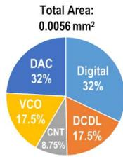
Figure 7.1.7: Experimental setup, chip photo and breakdown of total area.
