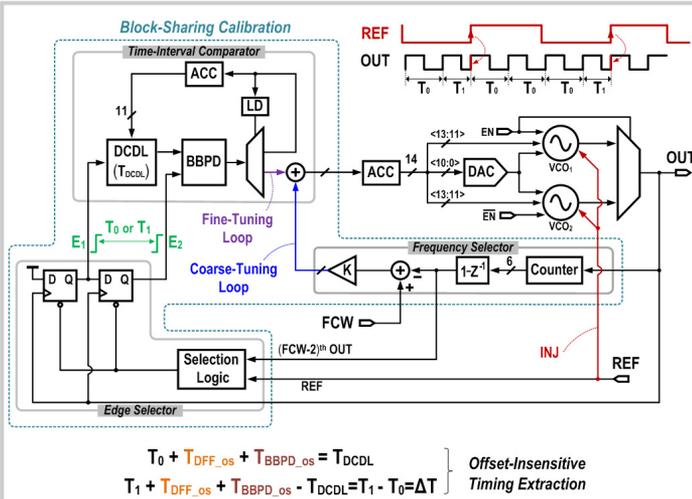
Figure 7.1.1: Proposed all-digital MDLL with a block-sharing FTL for better area and power efficiency. Edge re-extraction equalizes the periods  $T_0$  and  $T_1$  of OUT, being immune to the timing offset in the DFF ( $T_{DFF\_os}$ ) and BBPD ( $T_{BBPD\_os}$ ).
