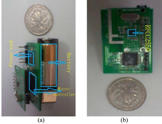
Figure 3. The bio-signal acquisition device in (a) lateral view (b) front view
