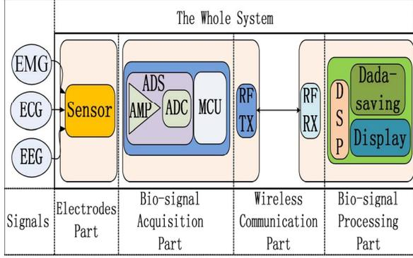
Figure 2. Block diagram of the data acquisition system
